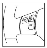
The cruise control buttons are located on the steering wheel. (S) **(On/Off):** Press this button to turn the cruise control system on and off. There is a indicator light on the button that will come on when cruise control is active.
